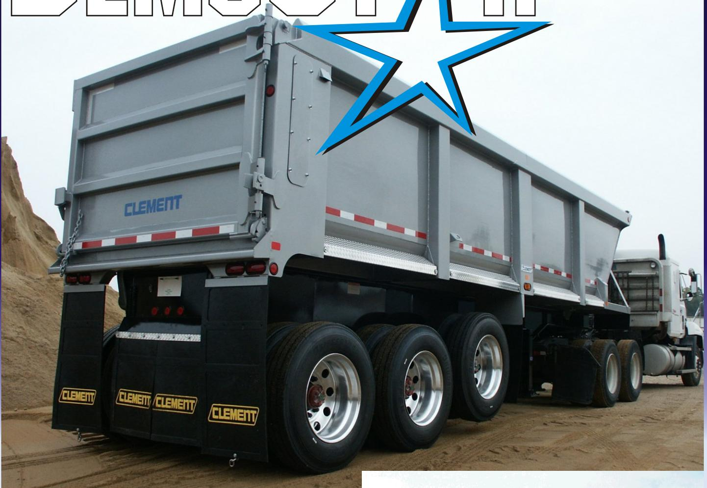
*The DemoStar's rugged barn door tailgate of 1/4-inch AR450 steel is supported by extra heavy-duty hinges. 1-1/8-inch greaseable hinge pins and 1-1/2-inch latch bars assure long, low maintenance operation.*
